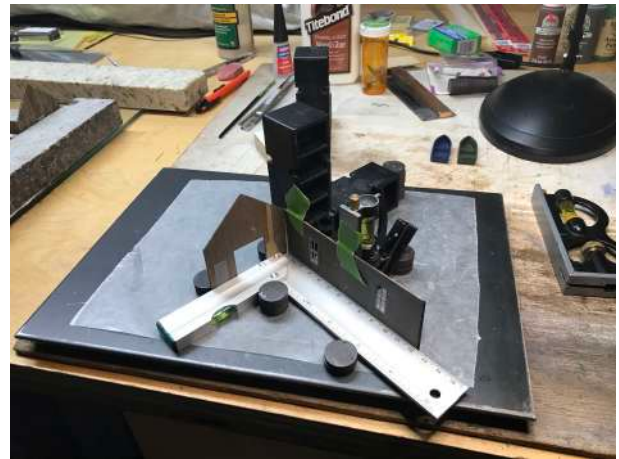
Step 2: front wall & side wall in alignment jig while bonding corner joint
