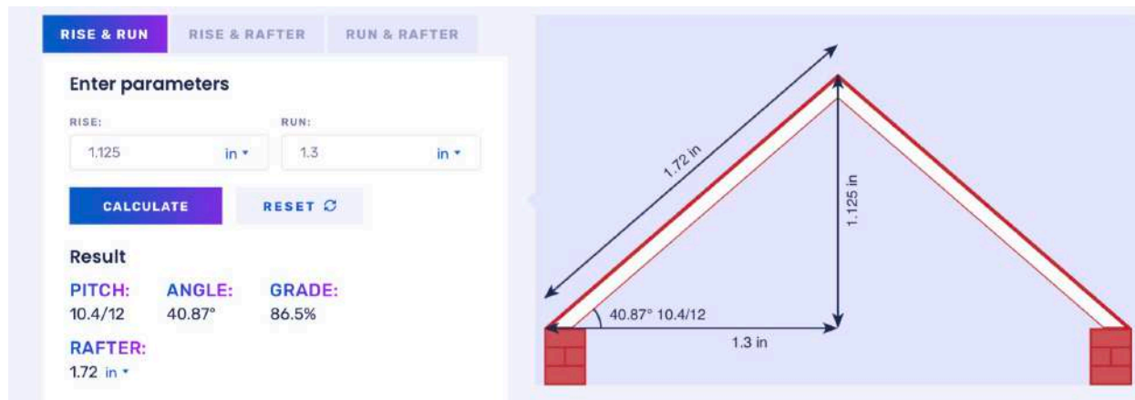
Roof pitch & rafter calculation
