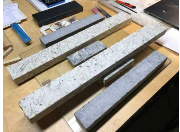
A wall section with freshly glued bonded siding boards is beneath each granite weight
