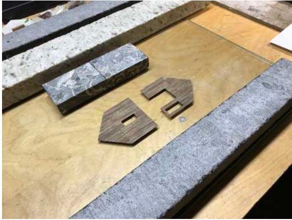
Granite weights used to flatten front and back walls with freshly glued siding boards
