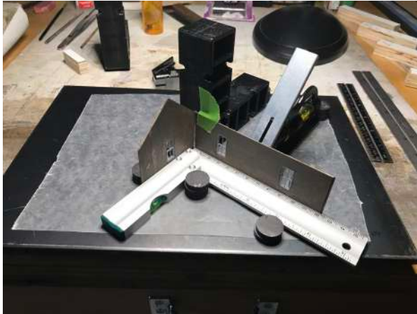
Step 1: back wall & side wall in alignment jig while bonding corner joint
