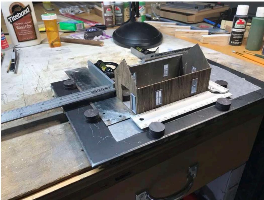
Step 3: wall sub-assemblies in alignment jigs while bonding corner joints
